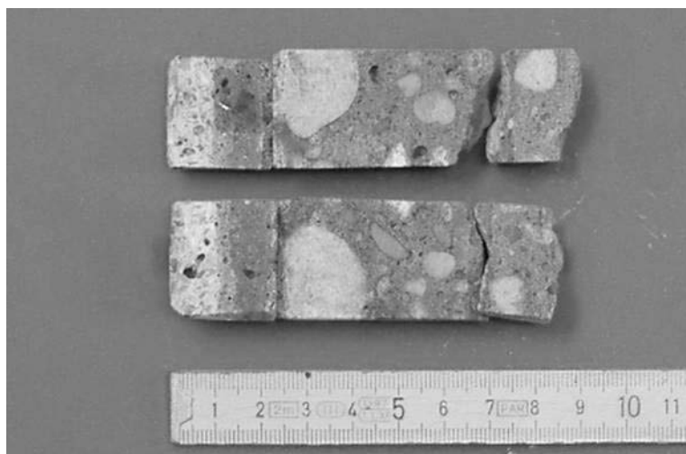
Figure 17 - Phenolphthalein test on a core extracted from a main pilaster.
