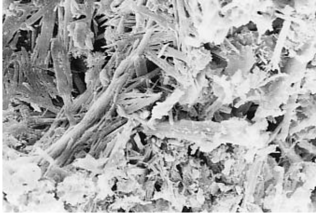
Figure 5 - Enlarged cement-gel particle, as observed by means of an electron microscope.
