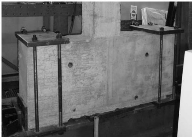
Figure 2 - View of the bottom part of a column and of the foundation block anchored to the strong floor.
