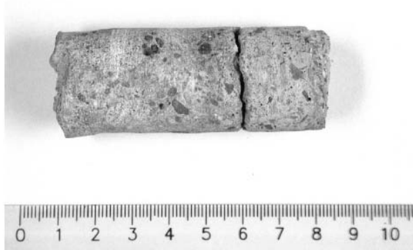
Figure 13 - Example of a core (MAPEI Report, 2007).
