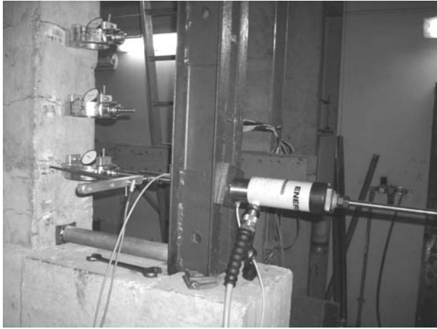
Figure 11 - Test rig for the pull-out tests.
